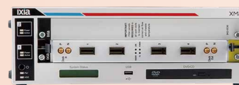
IXIA 400GbE Jumpstart Test System
